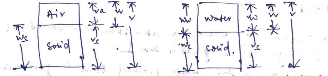
(two phase of soil element in dry state & saturated state)
