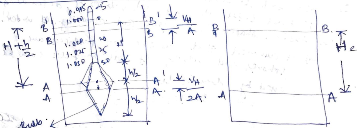
1. A hydrometer is an instrument used for the determination of the specific gravity of liquids.
