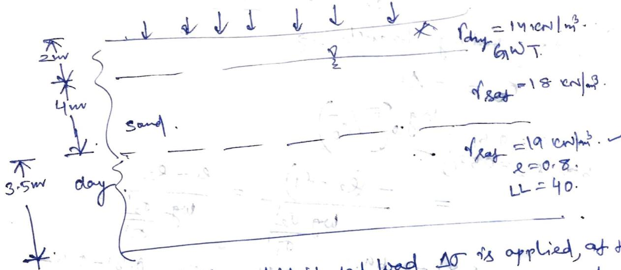
If the uniformly distributed load,  $\Delta \sigma$  is applied, at the ground surface, that is the settlement of the clay-layer caused by primary consolidation, if,
