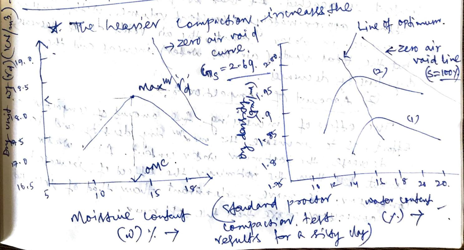
(compaction curves of Standard proctor Test and modified proctor test)
