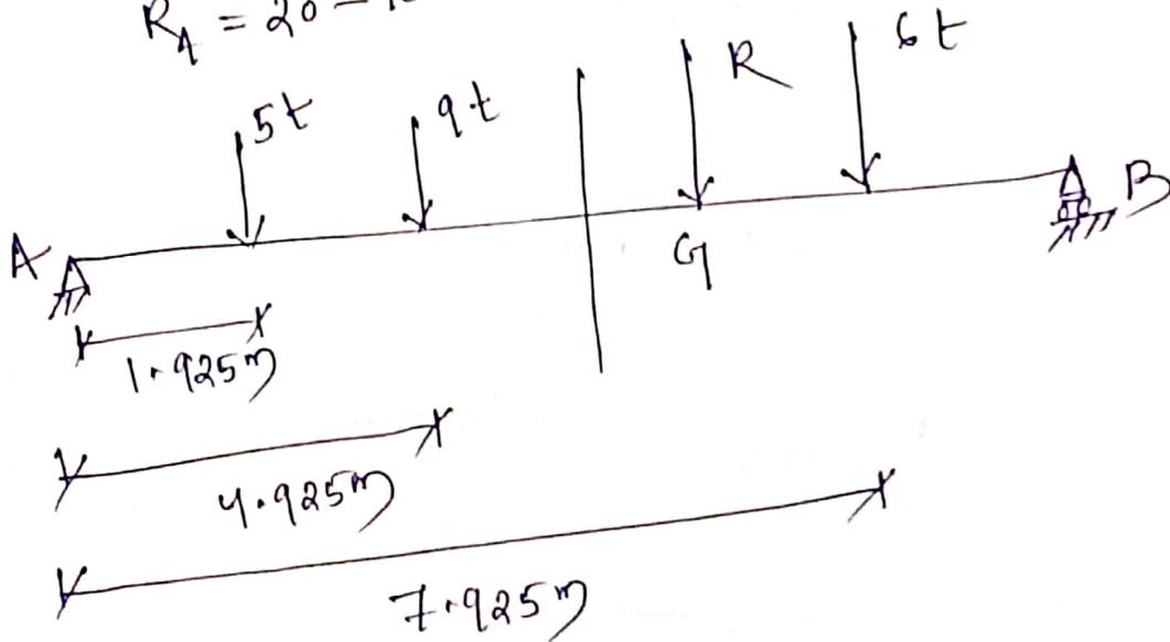
Absolute Max<sup>m</sup> B.M = B.M under Load  $9t$
