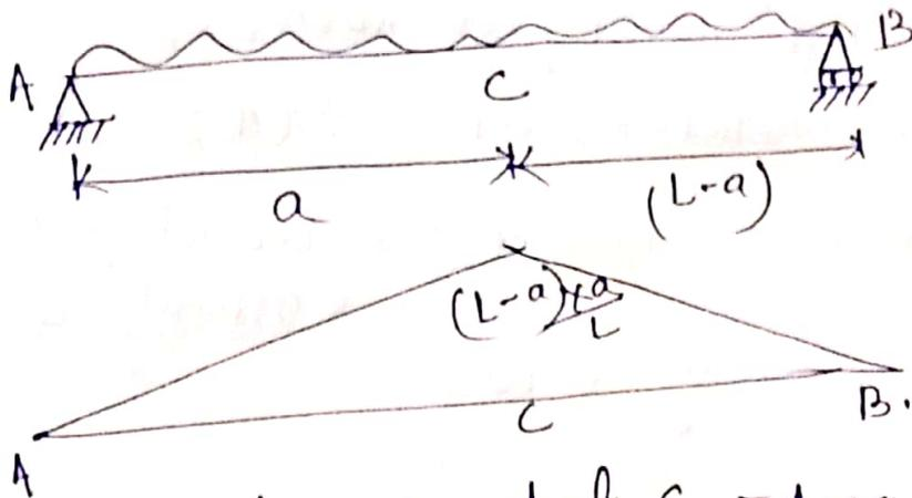
Maximum Bending Moment at C = Area of ILD for  $M_C \times w$
