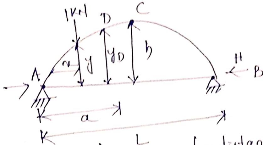
Consider a section  $x-x$  at a distance  $a$  from left support. At point  $D$ , the rise of point  $D$  is  $y_D$ .
