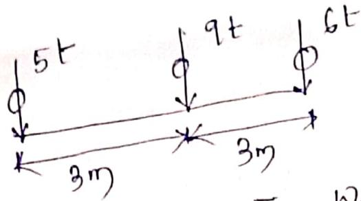
$$\text{C.G. of Load system} = \bar{x} = \frac{w_1 \bar{x}_1 + w_2 \bar{x}_2 + w_3 \bar{x}_3}{w_1 + w_2 + w_3}$$
