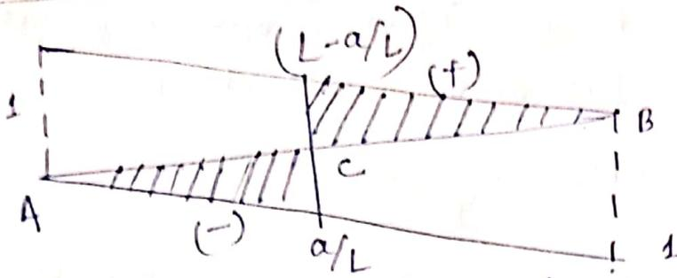
From the ILD, it is clear that Maximum positive shear force will occur when the Load is just to the right of section c.
