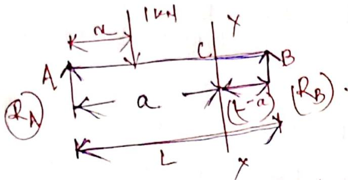
Consider a simply supported beam and a unit load of 1 kN is at a distance of  $\alpha$  m from support A.
