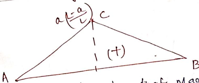
From the ILD it is clear that Maximum bending moment at c will occur when the Load is at the section itself.
