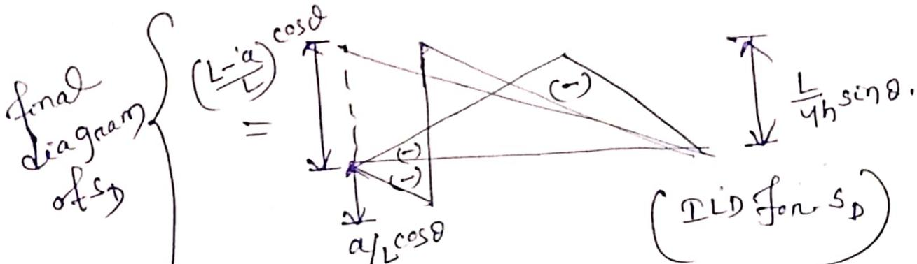
\* ILD for Normal thrust  $N_D$  is the combined diagram of (Beam shear)  $\times \sin \theta$  and ILD for  $H_D \times \cos \theta$
