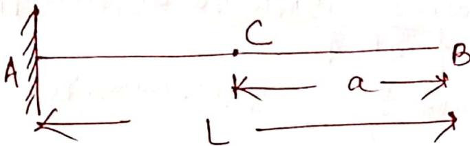
Consider a cantilever beam AB in which point C is there at a distance 'a' from support B.
