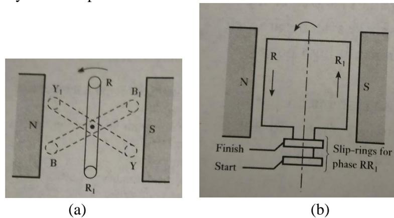
Fig. 2.1 (a) Generation of three phase emfs and (b) Loop  $RR_1$  at the instant of maximum emf with positive direction of voltages in coil sides.
