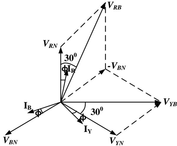
Fig. 2.16 Phasor diagram for balanced star connected load
