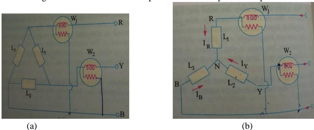
Fig. 2.15 Connection diagram for measurement of power by two wattmeter method for (a) delta connected load (b) star connected load
