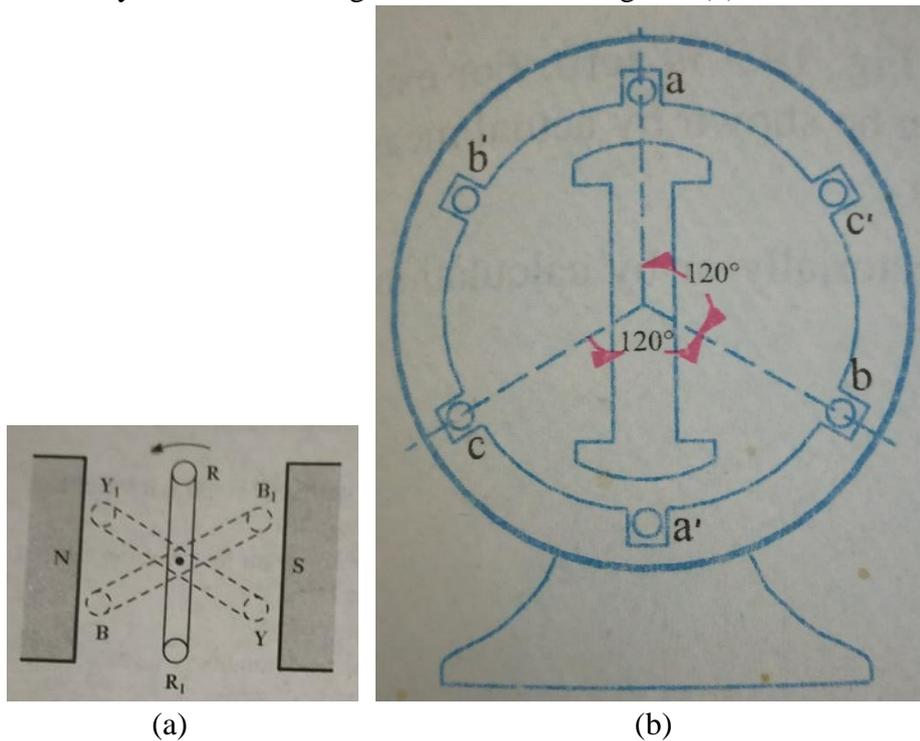
Fig. 2.3 Generation of three phase emfs (a) stationary field and rotating coils, (b) stationary coils and rotating field
