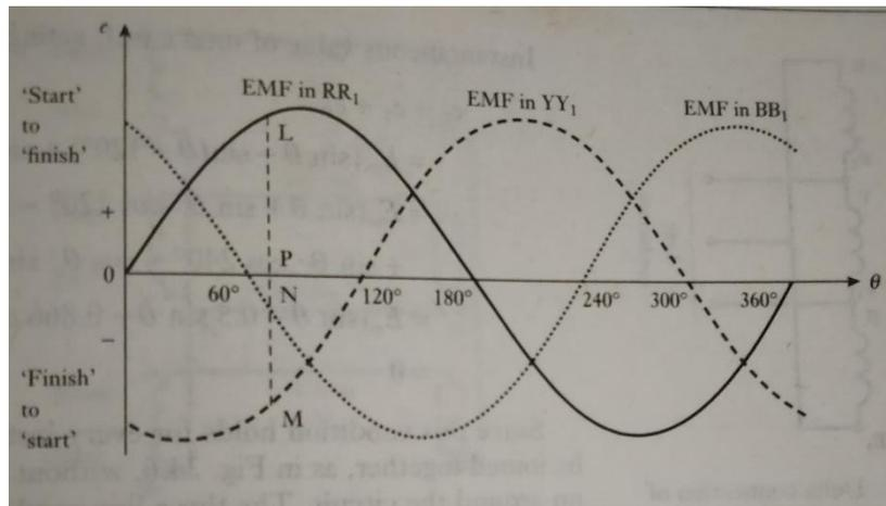
Fig. 2.2 Waveforms of three-phase emfs.
