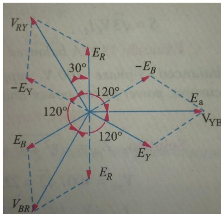
Fig. 2.11 Phasor diagram for computation of line voltage in star connection.
