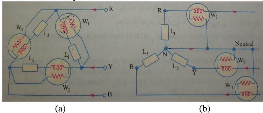
Fig. 2.14 Connection diagram for measurement of power by three wattmeter method for (a) delta connected load and (b) star connected load.
