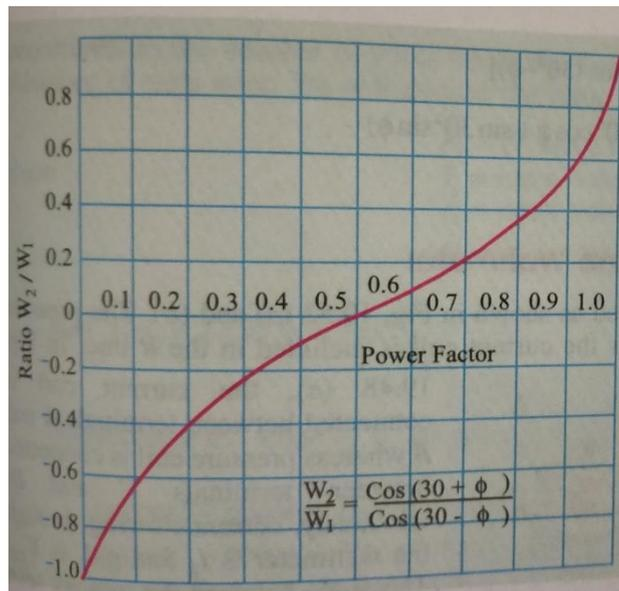
Fig. 2.17 Watt-ratio curve
