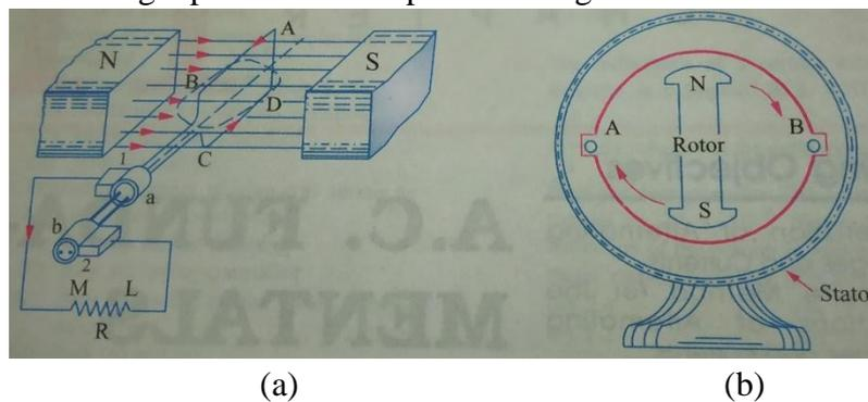
Fig. 2.4 Generation of single phase emf (a) stationary field and rotating coils, (b) stationary coils and rotating field
