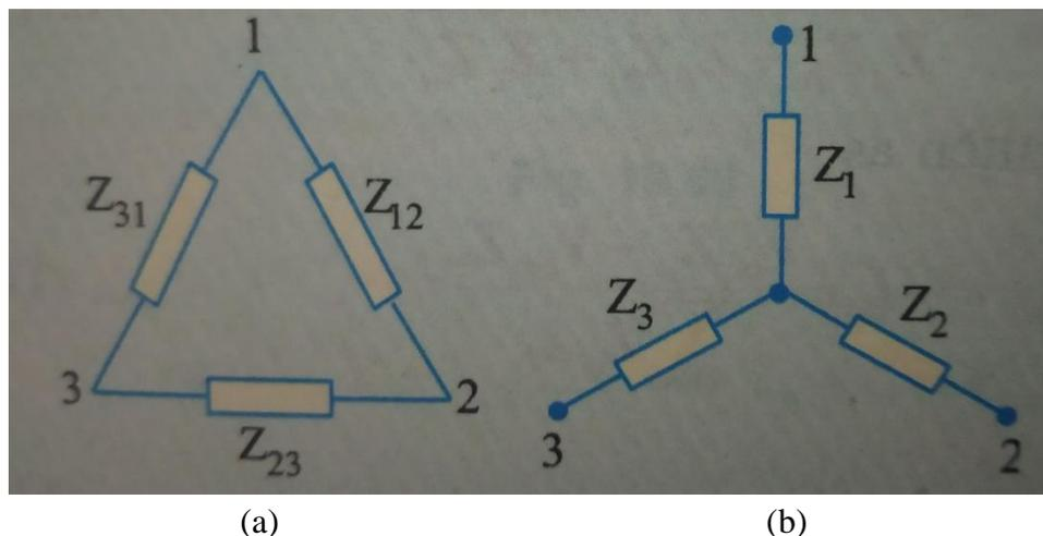
Fig. 2.18 Delta/Star and Star/Delta Conversion (a) Delta connected load and (b) Star connected load
