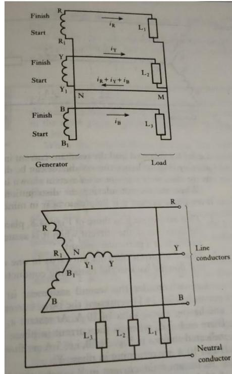
Fig. 2.8 Star connection of three phase windings (Three-phase four wire system)
