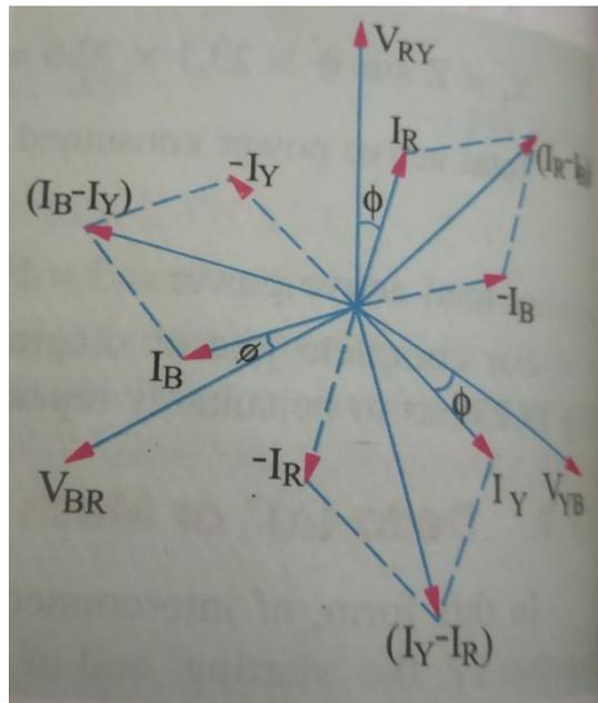
Fig. 2.13 Phasor diagram for computation of line current in delta connection
