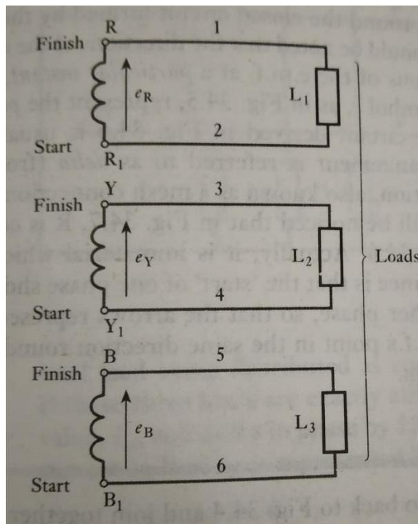
Fig. 2.5 Three phase windings with six-line conductors.
