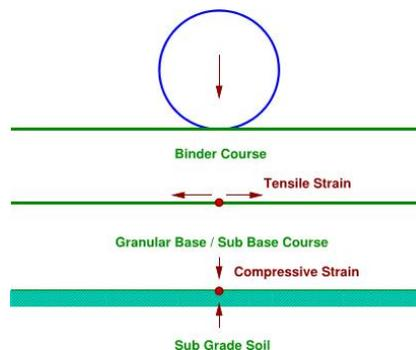
Fig. 33.1 Critical Locations in Pavement
