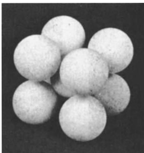
Fig.4. Hard-ball model of the body-centered cubic unit cell
