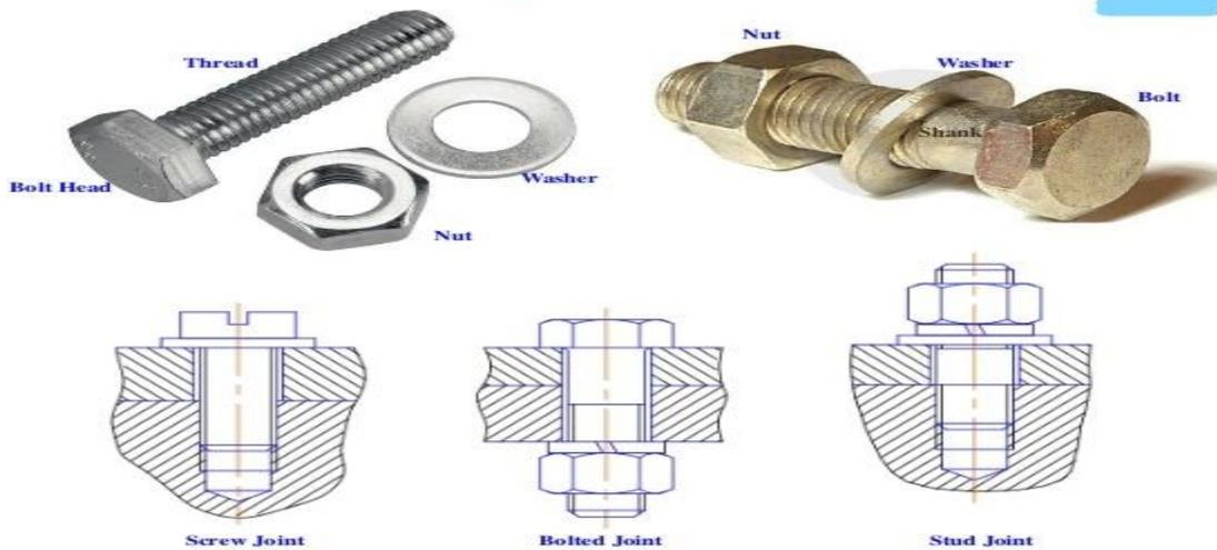
Components of a Bolted Joints 1. Bolt 2. Washer 3. (and/or) Nut . Different combinations of the above may be used for a joint depending on the load. 12.9 Class Bolt/Nut Means 12 . 9 ;  $12 \times 100 = 1200$  MPa is UTS  $9 \times 10 = 90\%$  of  $1200 = 1080$  MPa is YS Similarly for 10.9/8.8/4.4 etc
