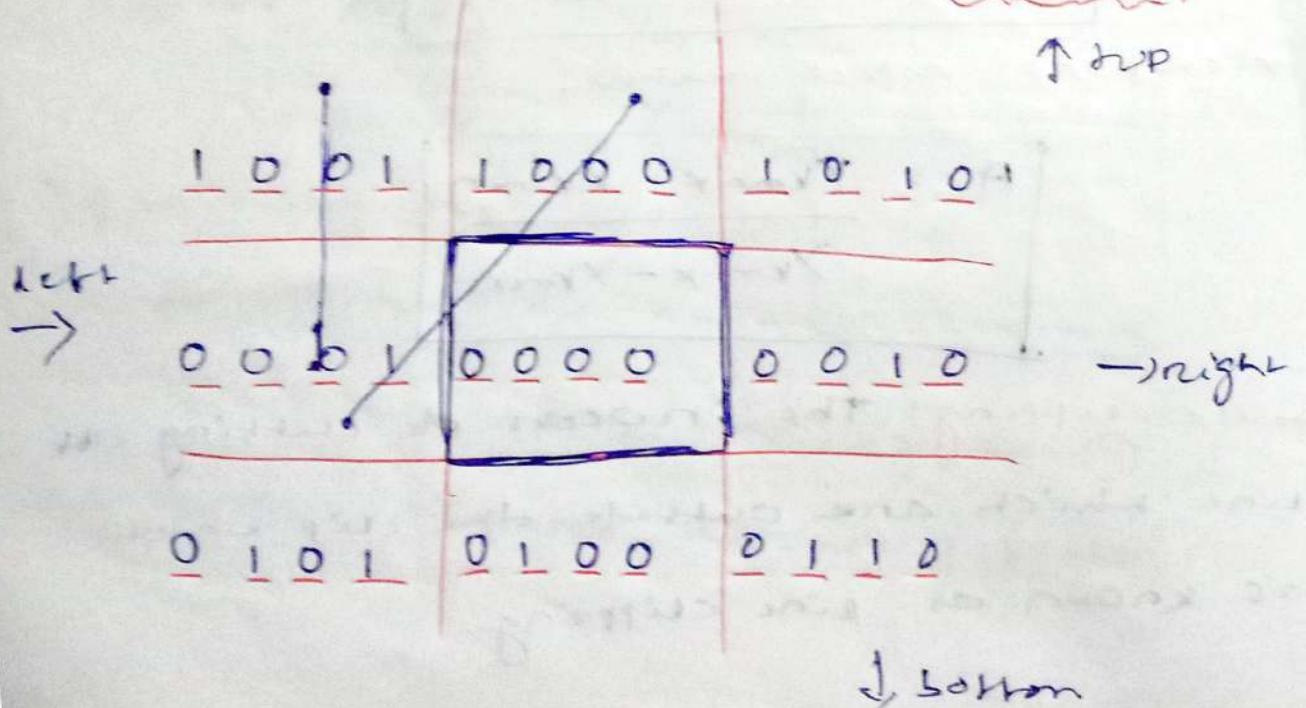
this algorithm uses 4-bit binary code for checking (the line) the location of the points relative to the boundary of the clipping rectangle.
