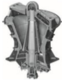
Fig.12 Cut section of Fuller-Traylor gyratory crusher (Courtesy FLSmidth Minerals).
