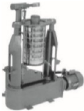
Fig.3 Ro-tap sieve shaker.
