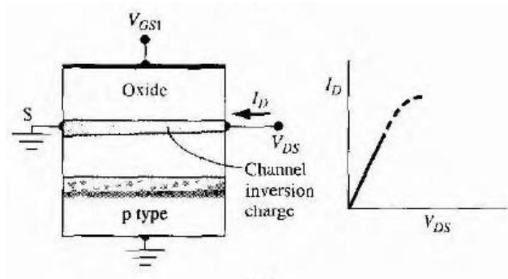
When  $V_{DS}$  increases to the point where the potential drop across the oxide at the drain terminal is equal to  $V_{TN}$ , the induced inversion charge density is zero at the drain terminal. This effect is schematically shown in Figure. At this point, the incremental conductance at the drain is zero, which means that the slope of the  $I_D$  versus  $V_{DS}$  curve is zero. We can write
