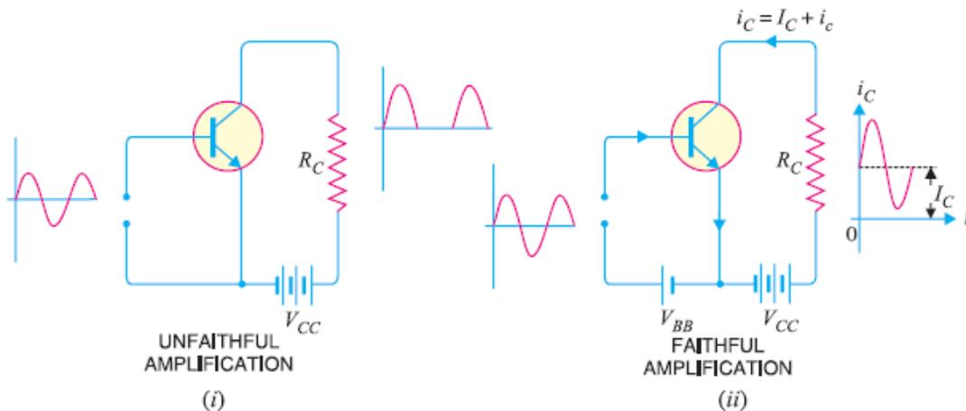
Now, introduce a battery source  $V_{BB}$  in the base circuit as shown in Fig. The magnitude of this voltage should be such that it keeps the input circuit forward biased even during the peak of negative half-cycle of the signal. When no signal is applied, a d.c. current  $I_C$  will flow in the collector circuit due to  $V_{BB}$  as shown. This is known as zero signal collector current  $I_C$ . During
