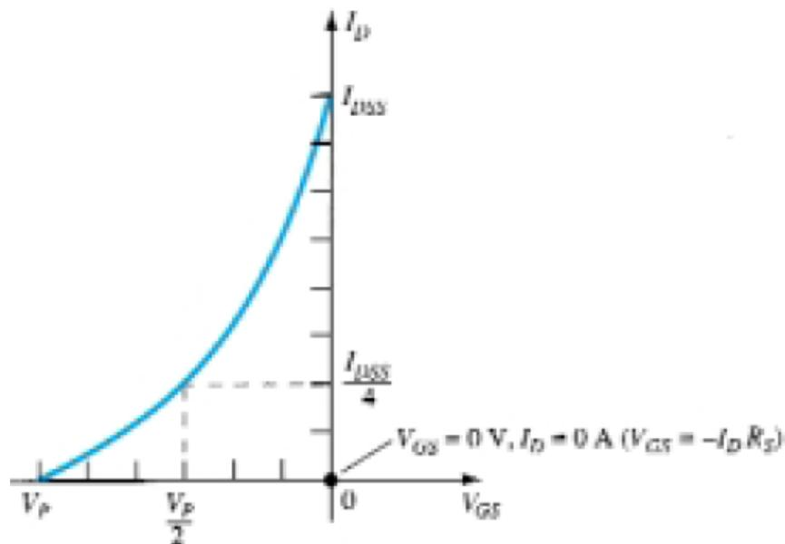
The second point for Eq. requires that a level of  $V_{GS}$  or  $I_D$  be chosen and the corresponding level of the other quantity be determined using Eq. The resulting levels of  $V_{GS}$  and  $I_D$  will then define another point on the straight line and permit an actual drawing of the straight line. Suppose, for example, that we choose a level of  $I_D$  equal to one-half the saturation level. That is,
