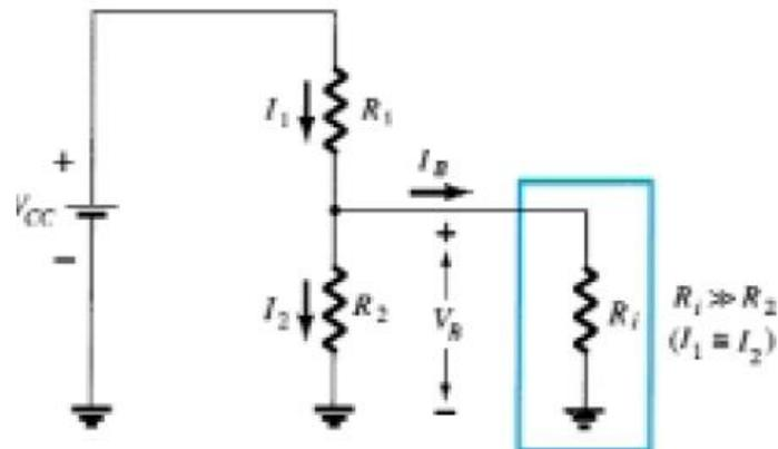
The voltage across  $R_2$ , which is actually the base voltage, can be determined using the voltage-divider rule (hence the name for the configuration). That is,
