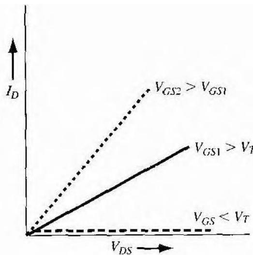
When  $V_{GS} < V_{TN}$ , the drain current is zero. As  $V_{GS}$  becomes larger than  $V_{TN}$ , channel inversion charge density increases, which increases the channel conductance.
