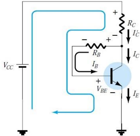
From the circuit diagram shown in Figure, applying Kirchoff's voltage law to the input circuit, we have
