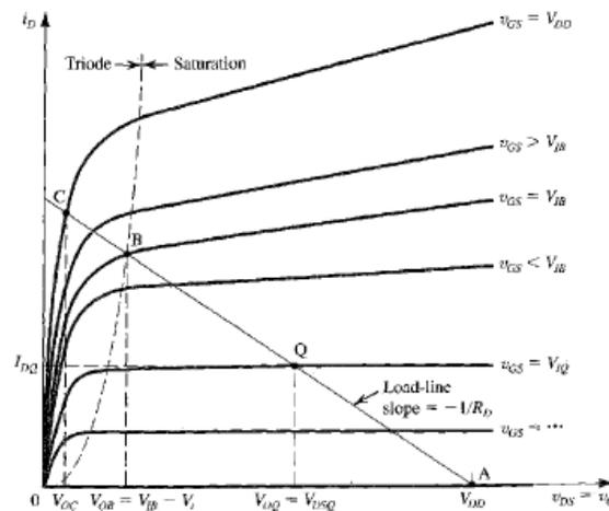
The graphical construction of Fig. can now be used to determine  $v_0$  (equal to  $v_{DS}$ ) for each given value of  $v_I$  ( $v_{GS} = v_I$ ). Specifically, for any given value of  $v_I$ , we locate the corresponding  $i_D \sim v_{DS}$  curve and find  $v_0$  from the point of intersection of this curve with the load line.
