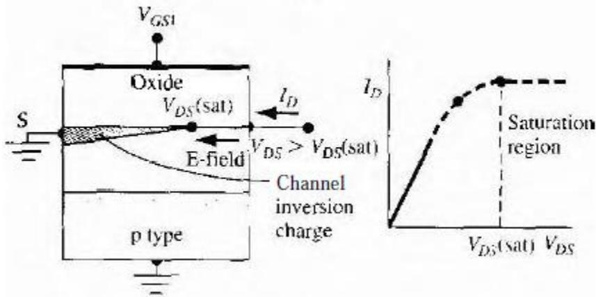
As the applied gate-to-source voltage changes, the  $I_D$  versus  $V_{DS}$  curve changes. The region for which  $V_{DS} < V_{DS}(sat)$  is known as the **non-saturation or triode region**. The ideal current-voltage characteristics in this region are described by the equation.
