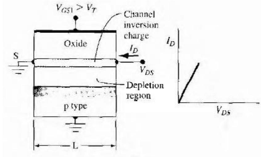
Figure shows the situation when the  $V_{DS}$  value increases. As the drain voltage increases, the voltage drop across the oxide near the drain terminal decreases, which means that the induced inversion charge density near the drain also decreases. The incremental conductance of the channel at the drain decreases, which means that the slope of the  $I_D$  versus  $V_{DS}$  curve will decrease. This effect is shown in the  $I_D$  versus  $V_{DS}$  curve in the figure.
