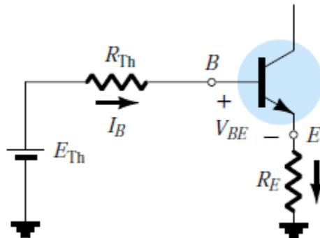
Applying KVL in the base-emitter loop
