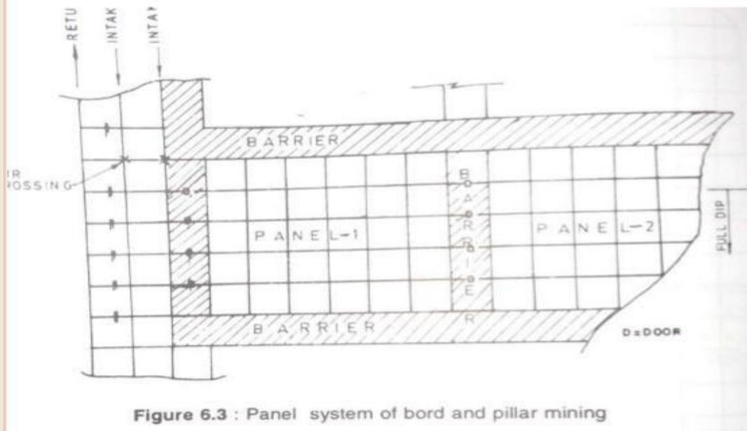
Figure 6.3 : Panel system of bord and pillar mining
