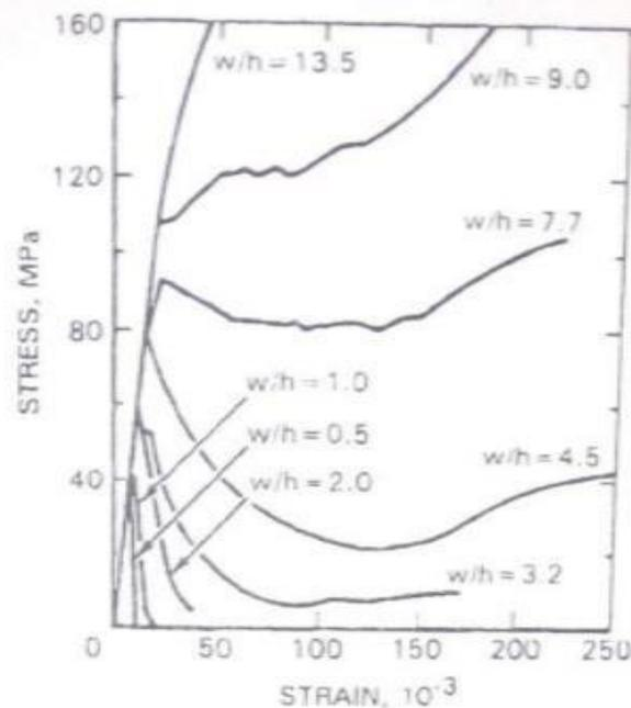
Figure 8.7 Complete stress strain curve for Indian coal specimen (Das, 1986)
