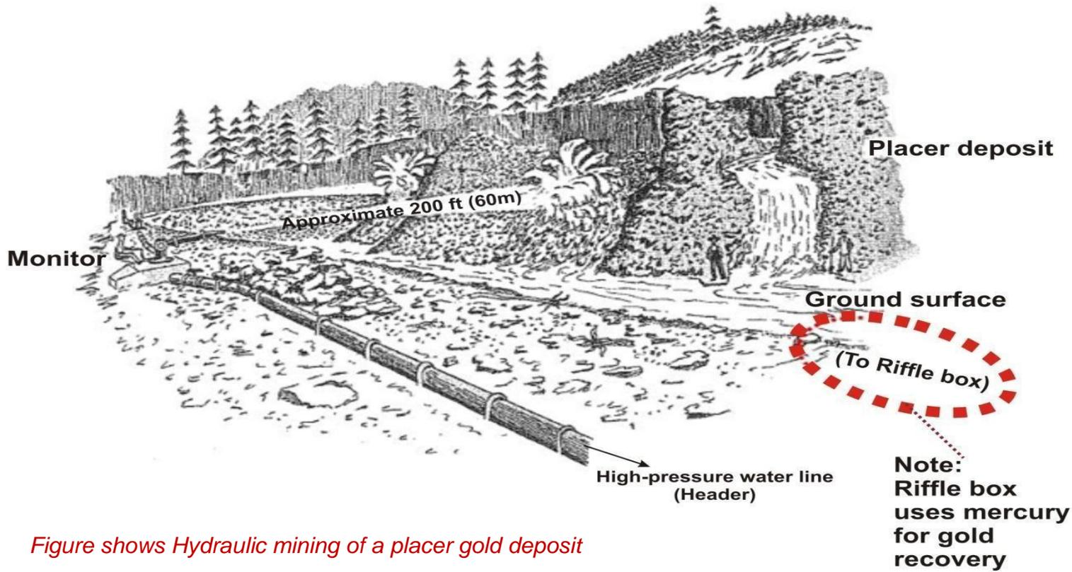
*Figure shows Hydraulic mining of a placer gold deposit*
