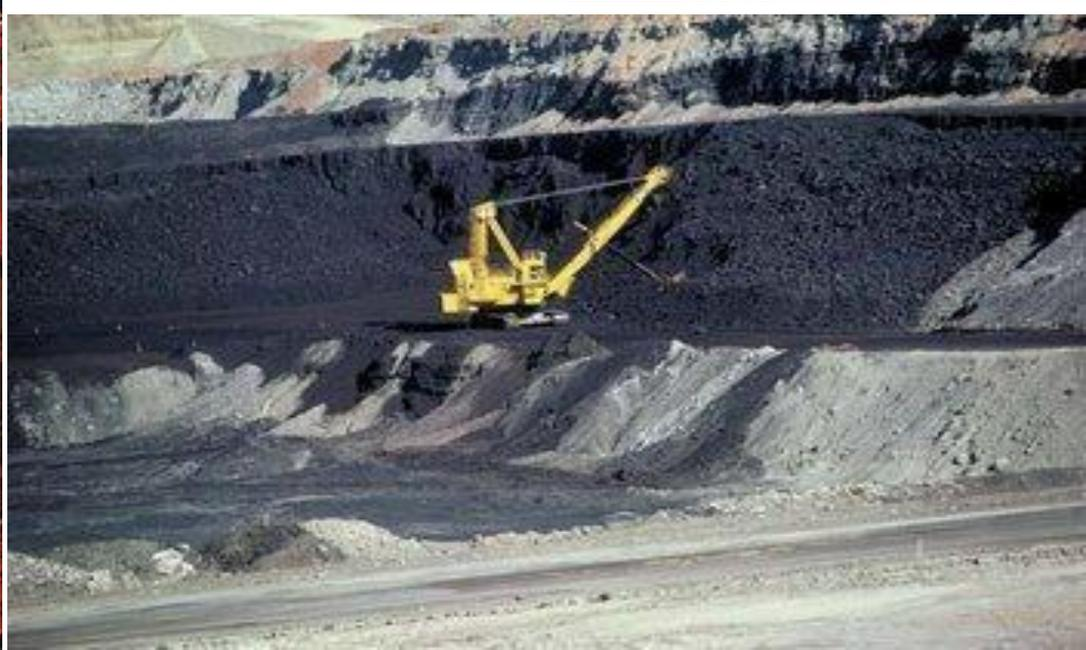
"Strip mining" is the practice of mining a seam of mineral by first removing a long strip of overlying soil and rock (the overburden). It is most commonly used to mine coal or tar sand. Strip mining is only practical when the ore body to be excavated is relatively near the surface.
