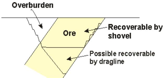
Massive deposit, high relief (Example copper sulphide).
