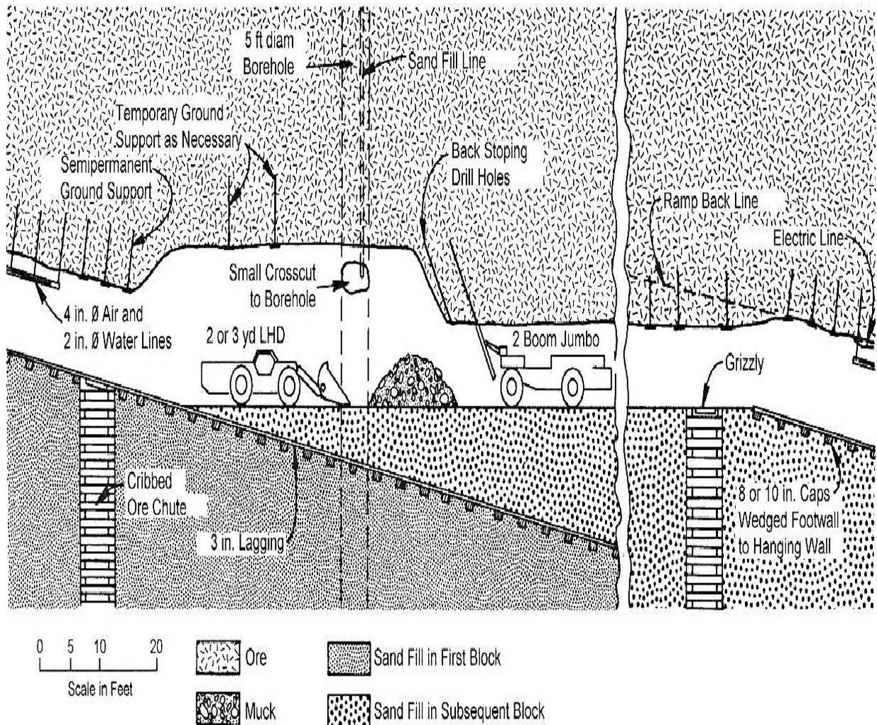
Figure: Cut-and-Fill Stopping Operation
