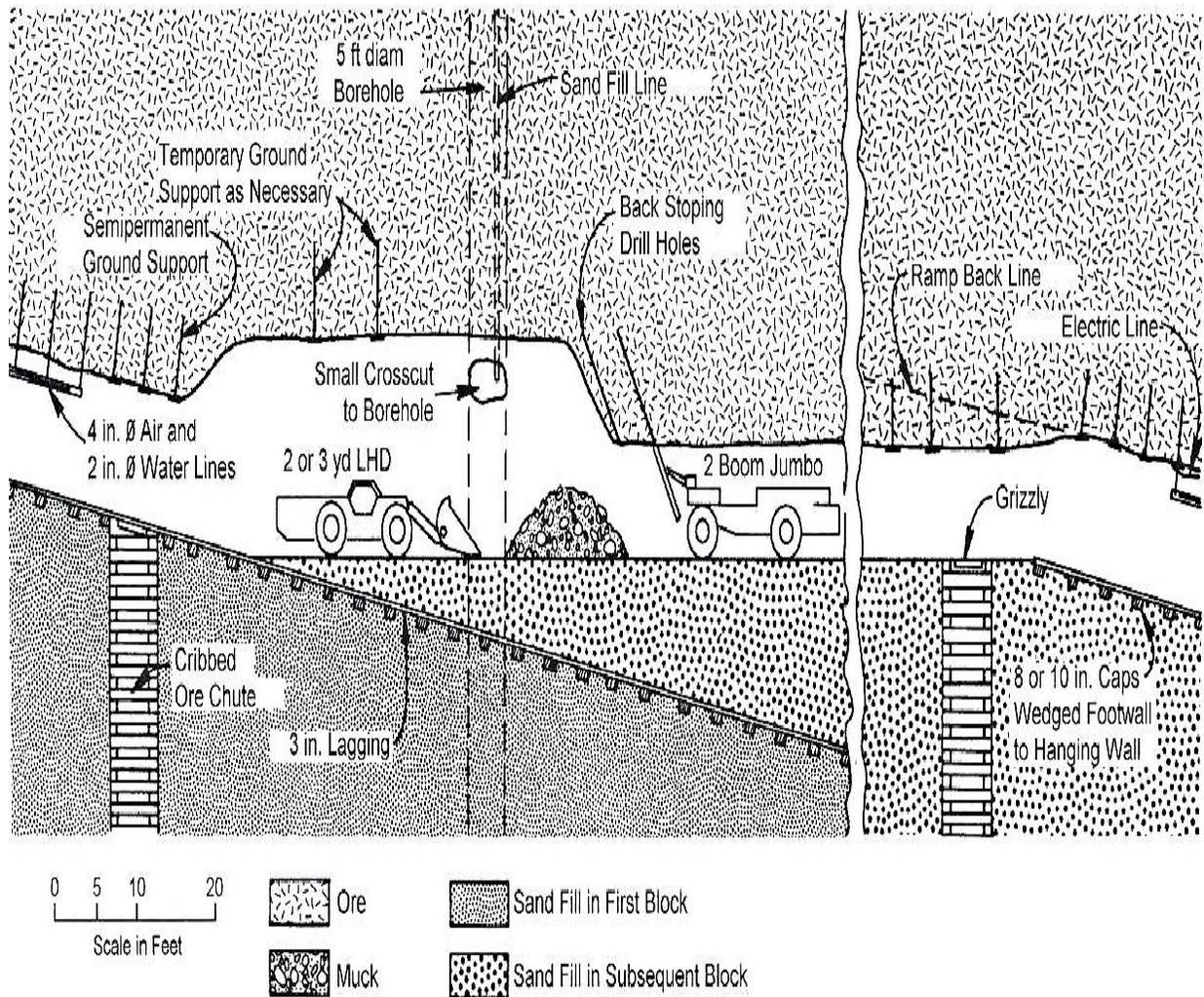
Figure: Cut-and-Fill Stopping Operation
