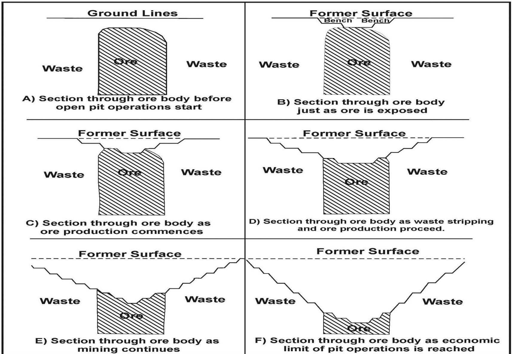
*Figure: Open-pit mining sequence (for pipe-like orebody)*
