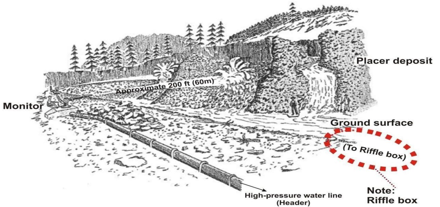
*Figure shows Hydraulic mining of a placer gold deposit*
