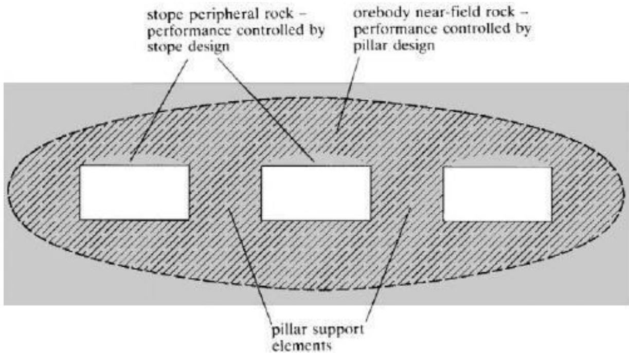
Schematic illustration of problems of mine near-field stability and stope local stability, affected by different aspects of mine design
