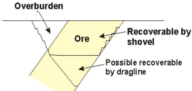
Massive deposit, high relief (Example copper sulphide).
