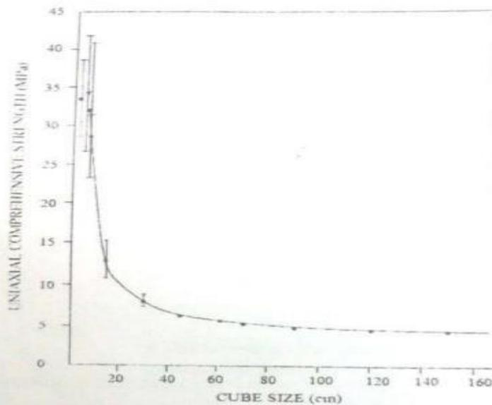
**Figure 8.6:** The relationship between the size and the strength of the specimen (Bieniawski, 1968)
