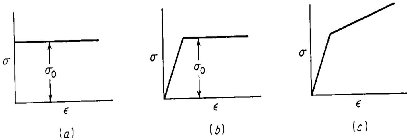
**Figure 3-2** Idealized flow curves. (a) Rigid ideal plastic material; (b) ideal plastic material with elastic region; (c) piecewise linear (strain-hardening) material.
