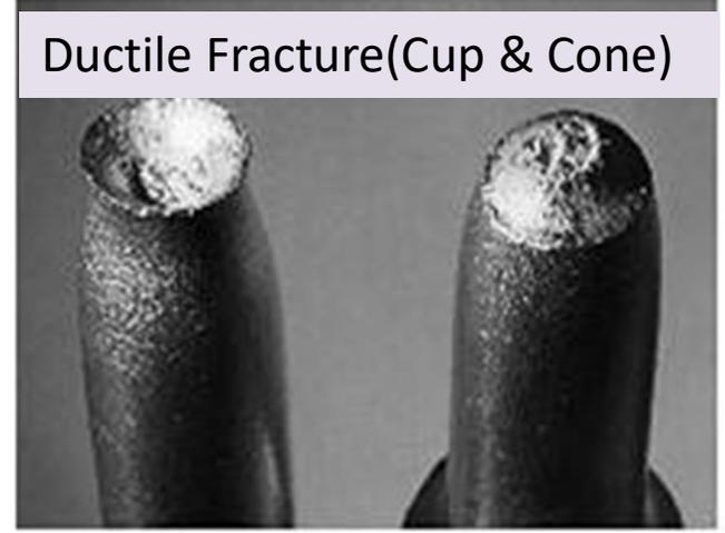
Ductile Fracture(Cup & Cone)
