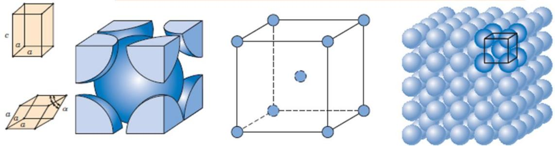
**BCC unit cell & aggregate of atoms**
