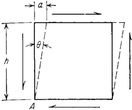
Figure 1-7 Shear strain.
