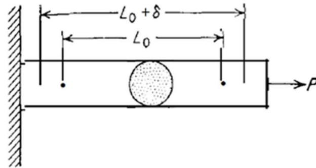
Figure I-I Cylindrical bar subjected to axial load.
