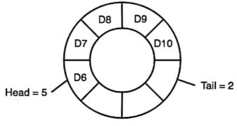
In such a situation the value of the Head pointer will be greater than the Tail pointer
