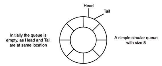
3. New data is always added to the location pointed by the rear pointer, and once the data is added, rear pointer is incremented to point to the next available location.
