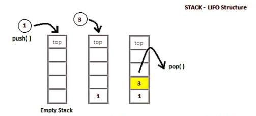
In a Stack, all operations take place at the "top" of the stack. The "push" operation adds an item to the top of the Stack.
