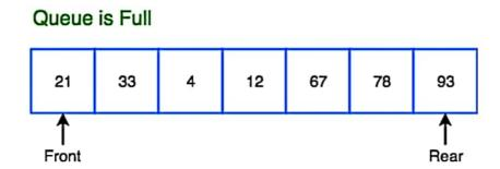
When we dequeue any element to remove it from the queue, we are actually moving the front of the queue forward, thereby reducing the overall size of the queue. And we cannot insert new elements, because the rear pointer is still at the end of the queue.
