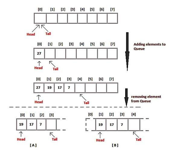
When we remove an element from Queue, we can follow two possible approaches (mentioned [A] and [B] in above diagram). In [A] approach, we remove the element at front position, and then one by one shift all the other elements in forward position.
