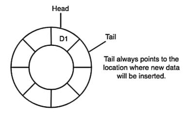
4. In a circular queue, data is not actually removed from the queue. Only the front pointer is incremented by one position when **dequeue** is executed. As the queue data is only the data between front and rear, hence the data left outside is not a part of the queue anymore, hence removed.
