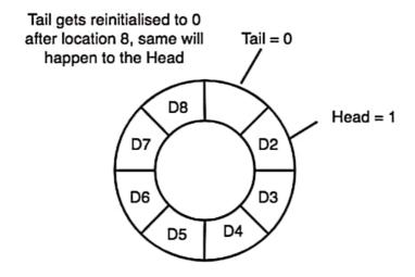
6. Also, the front and the rear pointers can cross each other. In other words, front pointer can be greater than the rear. Sounds odd? This will happen when we dequeue the queue a couple of times and the rear pointer gets reinitialised upon reaching the end of the queue.
