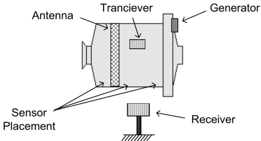
**(A Continuous Charge Measurement System)**
