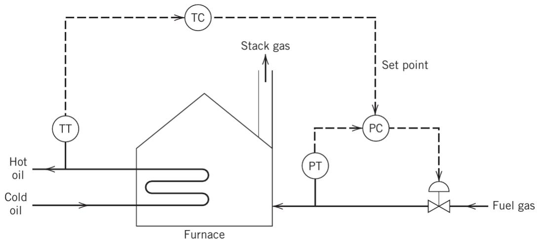
**(A furnace temperature control scheme using cascade control)**
