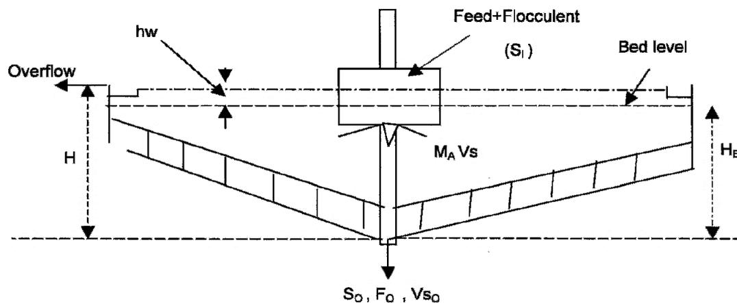
(Schematic diagram of thickener control)
