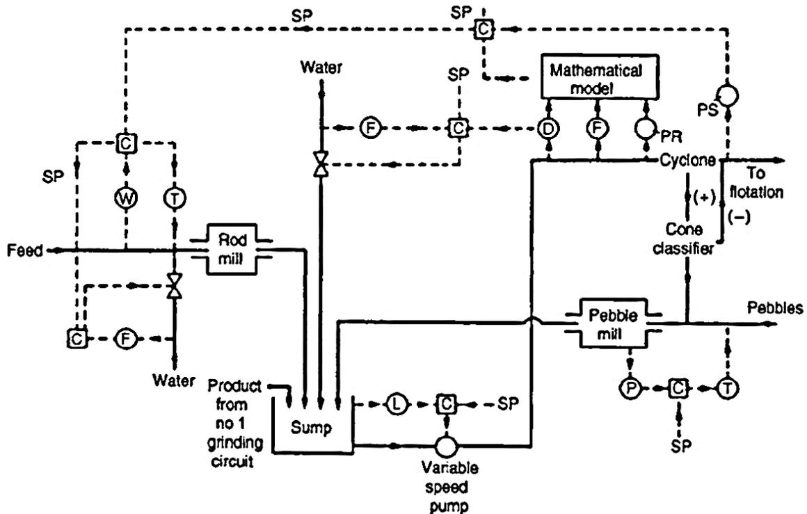
(A detailed grinding circuit control)
