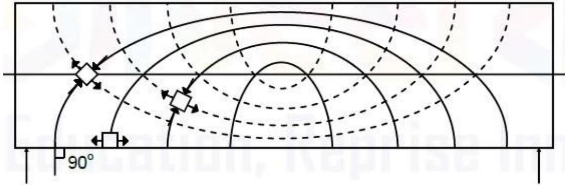
In a material like concrete which is weak in tension, tensile cracks would develop in a direction that is perpendicular to that of the principal tensile stress. Thus the compressive stress trajectories in the above figure indicate *potential* crack patterns, as shown below.
