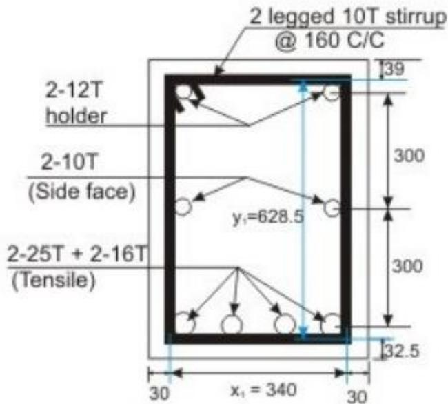
: Longitudinal (tension & side face) reinforcement of Prob. 1
