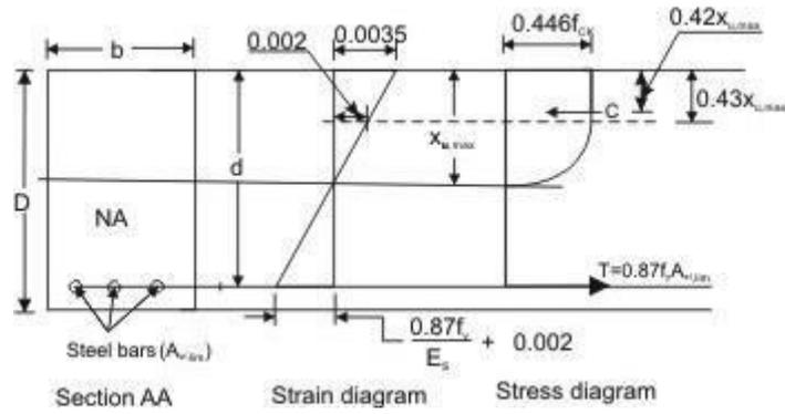
Rectangular beam under flexure  $x_u = x_{u,max}$
