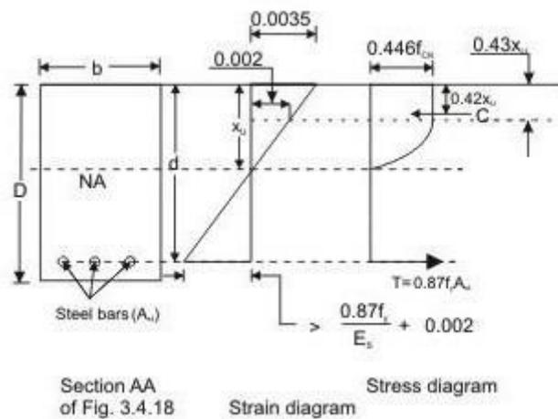
Rectangular beam under flexure
