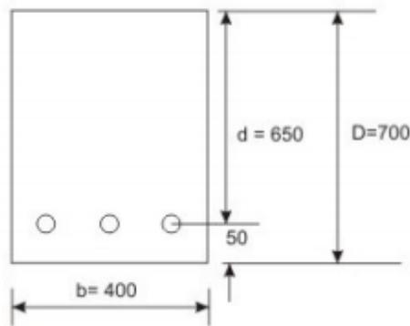
Determine the reinforcement required of a ring beam of  $b = 400$  mm,  $d = 650$  mm,  $D = 700$  mm and subjected to factored  $M_u = 200$  kNm, factored  $T_u = 50$  kNm and factored  $V_u = 100$  kN. Use M 20 and Fe 415 for the design.
