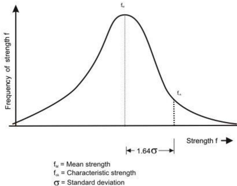
Figure shows frequency distribution curve of strength material (concrete or steel). The value of K corresponding to 5% area of the curve is 1.65.
