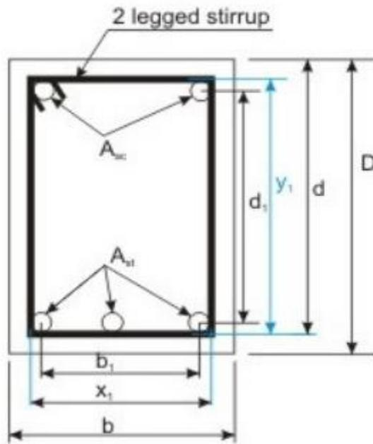
(d) The transverse reinforcement consisting of two legged closed loops enclosing the corner longitudinal bars shall be provided having an area of cross-section  $A_{sv}$  given below:
