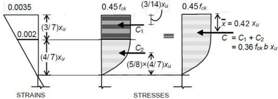
Fig. 1.9 Concrete stress-block parameters in compression
