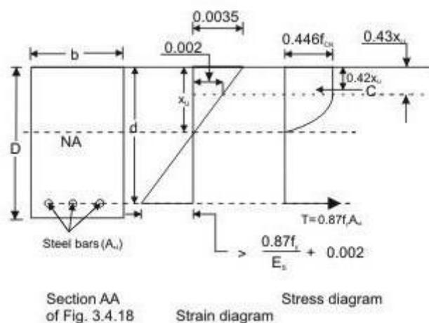
Rectangular beam under flexure
