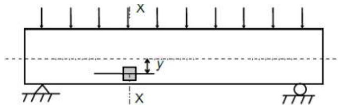
The combined flexural and shear stresses on that element can be resolved into equivalent *principal stresses*  $f_1$  and  $f_2$  acting on orthogonal planes.
