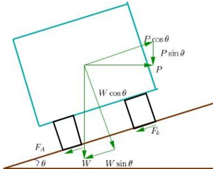
Fig.7.2 Analysis of super elevation
